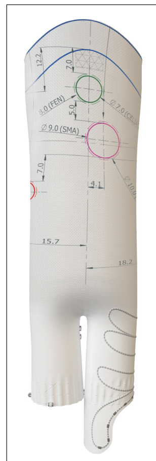
Figure 1. A representative device plan for a custom-made Fenestrated Anaconda™ Custom AAA Stent Graft System.
